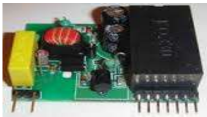
Gambar 1. KQ330 Power Line Carrier (PLC) modem
