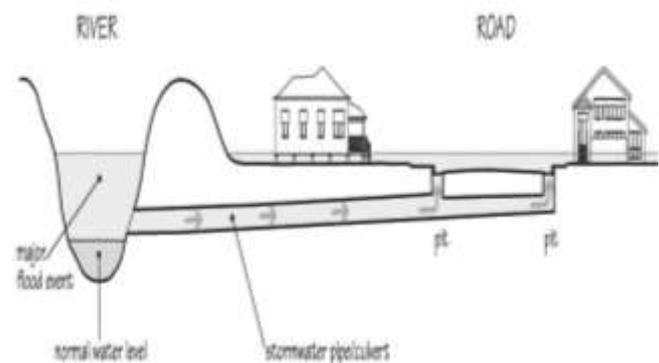
Figure 1. Backflow flooding concept [8]
