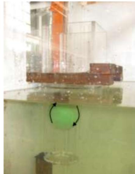
Figure 16: The ball spin and rotate due to upstream forces
