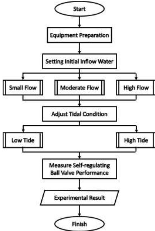
Figure 10. Experimental procedure
