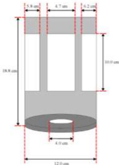
Figure 6. Cross Section Of The Floating Ball Mechanism
