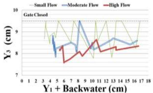
Figure 12. Performance of the floating ball mechanism related to inflow water
