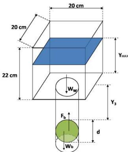
Figure 13. Acting forces to the floating ball mechanism
